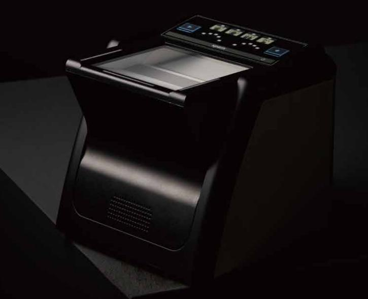
RealScan-G10 is a compact live-scanner for single and ten-print capture. Xperix's advanced optical technology allows high-speed image capturing and seamless image processing. IP65-rated dust and water resistant housing makes it suitable for indoor and mobile environments. With its proven reliability of FBI certification, RealScan-G10 is the perfect portable live-scanner for civil and criminal applications.
